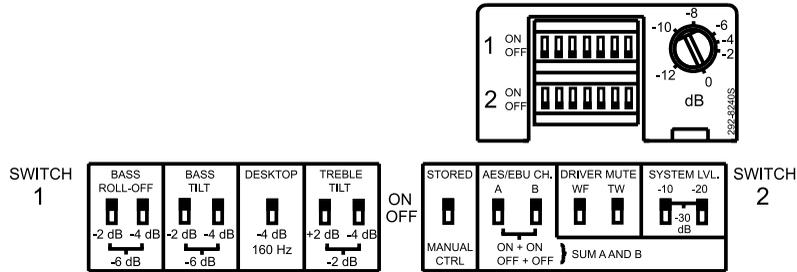
This feature is designed to compensate for the boost often occurring at this frequency range when the loudspeaker is placed upon a meter bridge, table or similar reflective surface.
